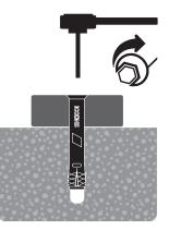
With correct size PH3 driver bit tighten anchor to specified torque. Installation complete!
